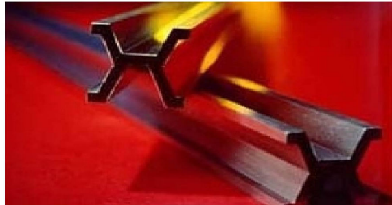
Figure: Historical International Prototype Meter bar, made of an alloy of platinum and iridium, that was the standard from 1889 to 1960.
